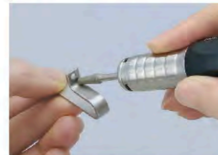
Tool : Electroplated Diamond Burs → Please see the NAKANISHI "POLISHING TOOLS" Catalog.
