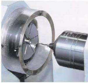
High rigidity and long clearance allow for high precision grinding of deep IDs.
